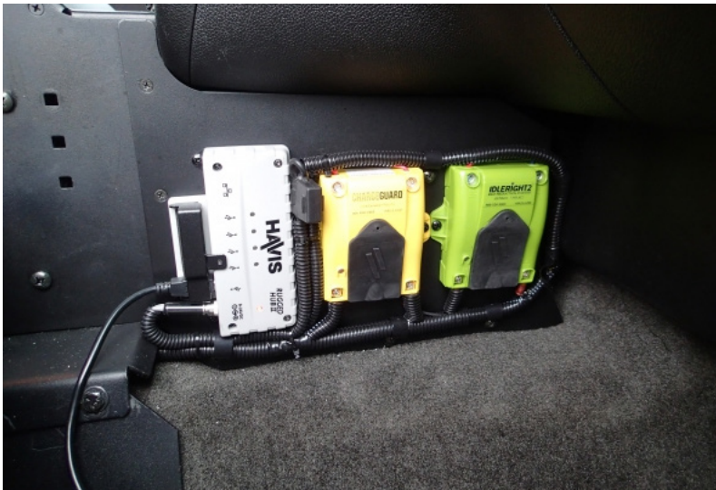
Figure 2: Havis IdleRight2 (green box) combined with a Havis Chargeguard (yellow box) and Hub (white box)
