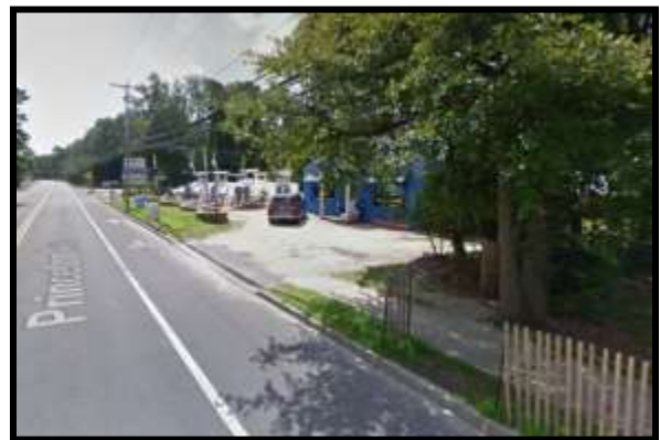
Figure 80: Sidewalk at Windward Beach Park ends abruptly at business area 300 feet away (Google Streetview)
