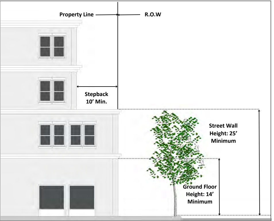
Figure D-4: REQUIRED STEP-BACK FOR ALL STREET-FACING FACADES ABOVE THE THIRD FLOOR
