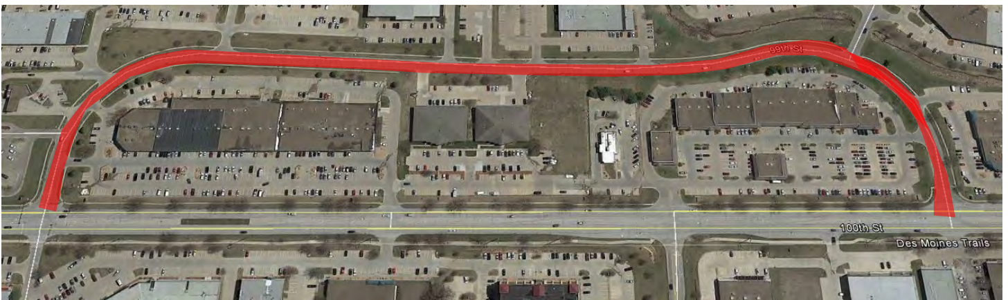
This is an example of a backage road in Urbandale, Iowa (highlighted in red). The backage road brings most traffic accessing the shopping centers off the main arterial road, eliminating all but two driveways onto the arterial. Many suburban shopping corridors would have one to two driveways for each center.
