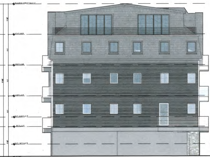
2 ELEVATION: SOUTH Scale: 1/8" = 1'-0"
