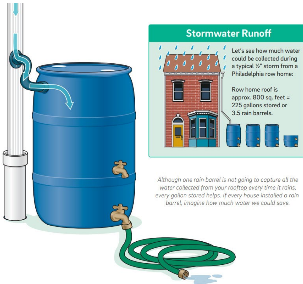
Figure 2. Rain barrel diagram from the Philadelphia Water Department.
