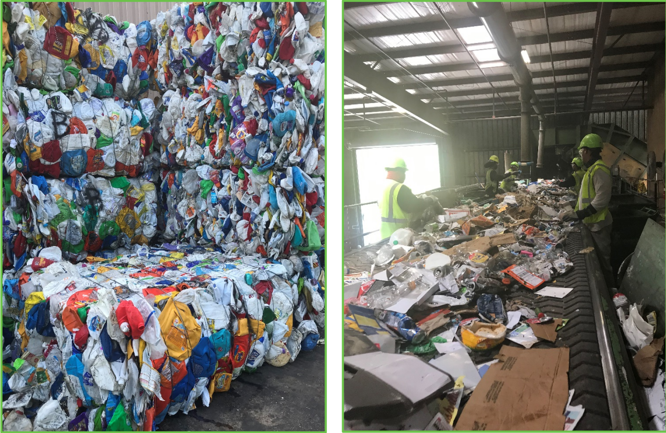
Figure 35. Waste processing facility showing compressed laundry bottles (left) and staff sorting non-recyclable or contaminated materials (right), Brevard County.
