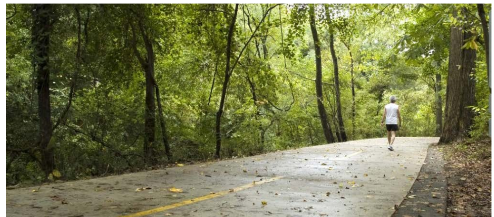
Tree root bridging allows the trail to come in close proximity to specimen trees without causing harm. A trail edge of porous concrete aids infiltration.
