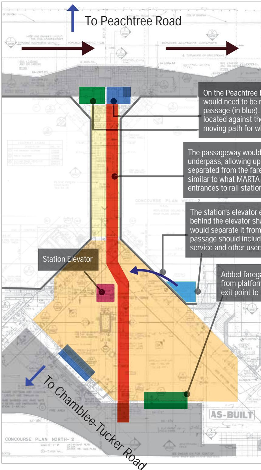
On the Peachtree Road station entrance, fare gates would need to be relocated to open an entryway for the passage (in blue). ADA-accessible gate would remain located against the passageway to allow a sufficient moving path for wheelchair users.
