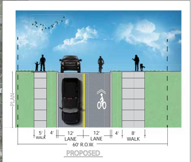
Due to existing street dimensions, the recommended treatment for this project is a shared-street connection for bicycles and expanded sidewalks (only one side currently has a four-foot attached sidewalk today).
