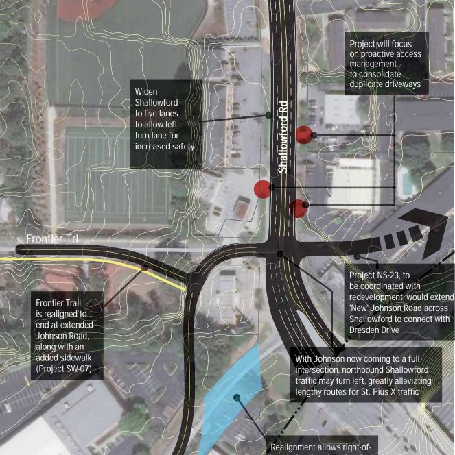
Realignment allows right-ofway to be abandoned and repurposed for other uses
