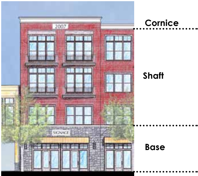
The diagram below illustrates how this style should be organized. Note the “heavier” material is placed beneath the “lighter” material.
