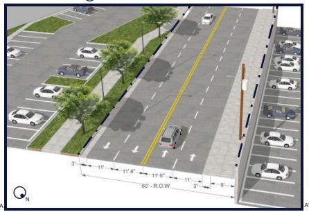
Figure 3.7g illustrates the existing condition of New Peachtree Road west of Hood Avenue. The R.O.W. is approximately 60'-wide with four travel lanes, two that are 11'-wide, two that are 11'-6"-wide, and power lines along the north side of the R.O.W. The south side of the road has a landscape buffer and a sidewalk that is outside the R.O.W. The north side of the road has a 9'-wide sidewalk.
