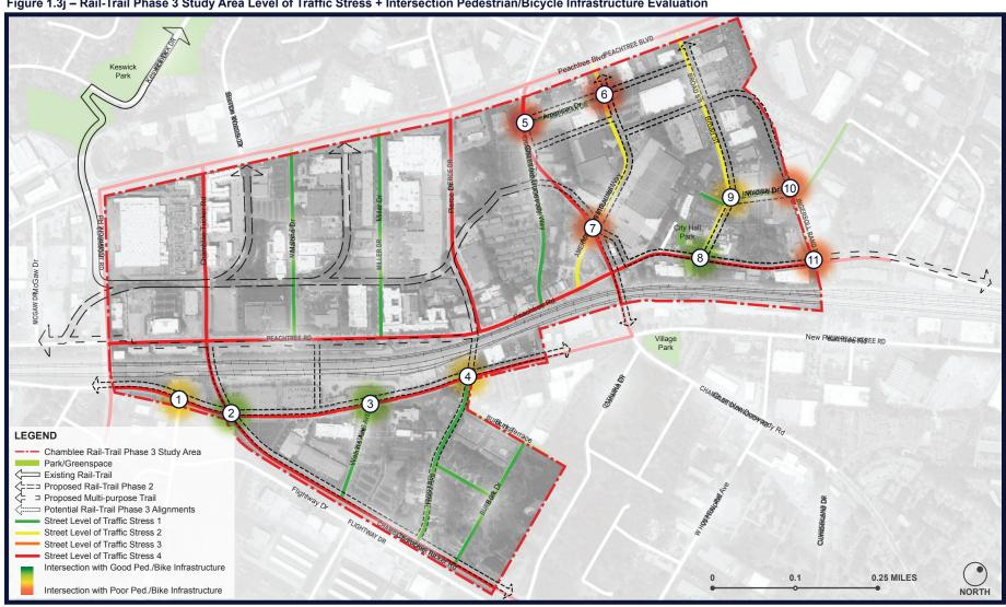
Figure 1.3j - Rail-Trail Phase 3 Study Area Level of Traffic Stress + Intersection Pedestrian/Bicycle Infrastructure Evaluation
