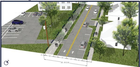
Figure 3.8c shows how the Rail-Trail could be implemented along Hood Avenue. The concept suggests adding a multipurpose trail along the west side of the road.
