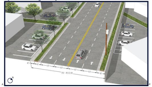
Figure 3.2c illustrates the existing condition of Chamblee Dunwoody Road. The R.O.W. is approximately 70'-wide with four 13'-wide travel lanes and power lines along the east edge of the R.O.W. There is one four-foot wide sidewalk on the west side of the street with no pedestrian connections to the east side of the street.
