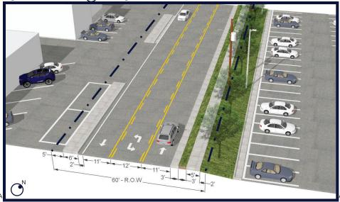
Figure 3.7e illustrates the existing conditions of New Peachtree Road east of Hood Avenue. The 60'R.O.W. contains three lanes, two that are 11'-wide and a center turn lane that is 12'-wide. The north side of the road is characterized by suburban style buildings and parking lots with multiple curb cuts. The south side of the road has less curb cuts and has power lines. 5' and 6'-wide sidewalks are located on the north and south sides of the road respectively.
