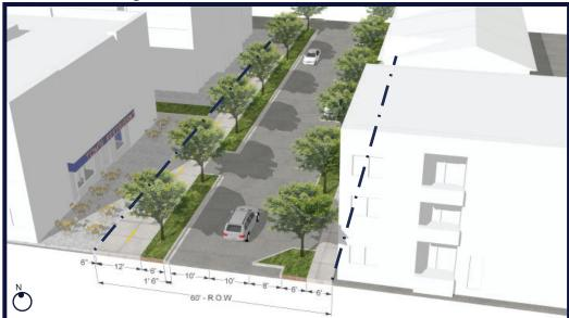
Figure 3.3f illustrates what a Phase 1 condition could look like along American Drive. Reducing the roadway width from 30' to 24'-wide allows sufficient space for the 12'-wide Rail-Trail and 6'-wide landscape buffer to be implemented on the north side of the street, which contains no power lines.
