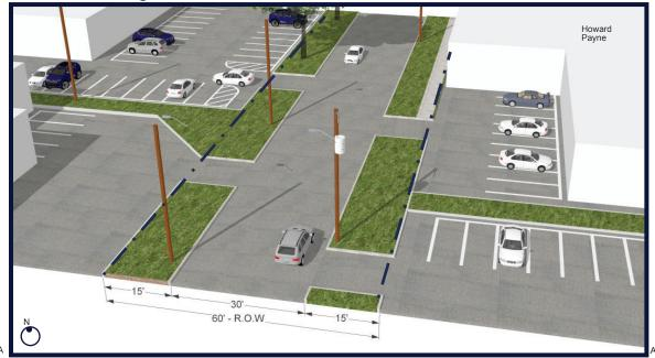
Figures 3.3f-3.3g illustrate an alternative alignment for the Rail-Trail between Chamblee Dunwoody Road and American Industrial Way along the American Drive R.O.W.
