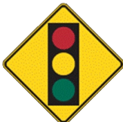
FIGURE 4-20 MUTCD Sign W3-3, Signal Ahead, 18" x 18"
