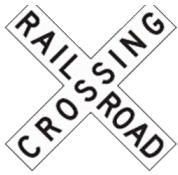
FIGURE 4-17 MUTCD Sign R15-1, Grade Crossing (Crossbuck), 24" x 4.5"
