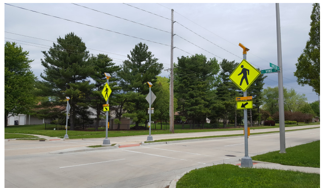
FIGURE 4-44 Median refuge island and RRFB on Windsor Road at Vine Street
