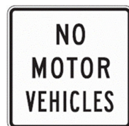
FIGURE 4-16 MUTCD Sign R5-3, No Motor Vehicles, 24" x 24"
