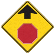
FIGURE 4-18 MUTCD Sign W3-1, Stop Ahead, 18" x 18"
