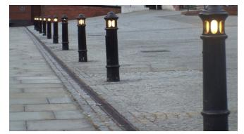
Example of bollard lights used to illuminate and protect pedestrian areas
