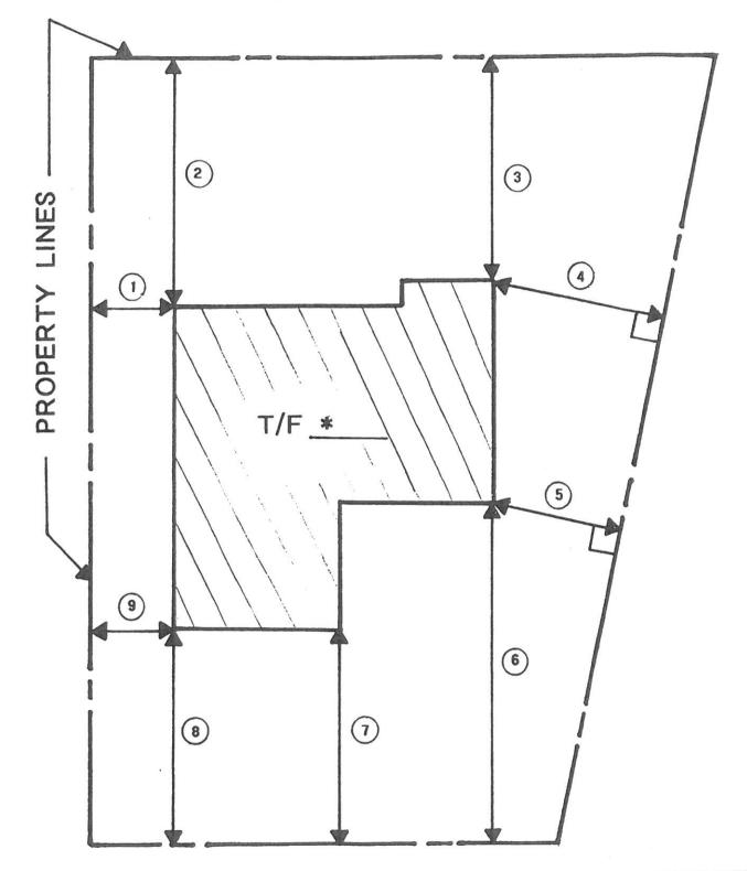
\* INDICATE THE LOCATIONS AND ELEVATIONS FOR ALL STEPS IN THE TOP OF FOUNDATION.
