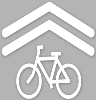
TYPICAL PAVEMENT MARKING
