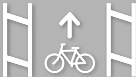
TYPICAL PAVEMENT MARKING
