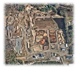
Loureiro used a fixed wing drone to fly the site and completed the field activities in about six hours. The related mapping was processed and a final existing conditions plan was ready for use within four days.
