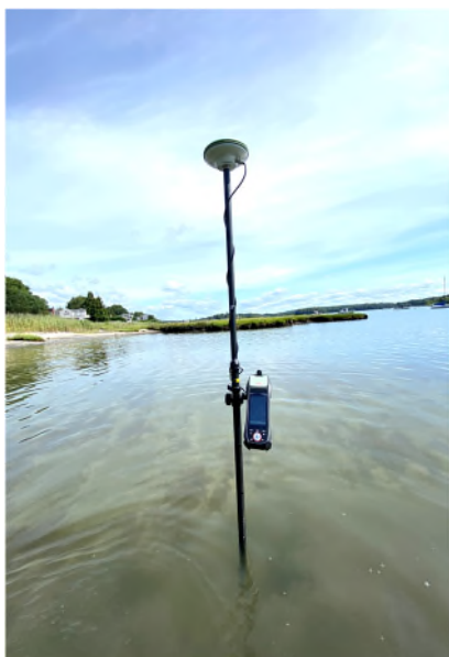
RTK GPS used to determine substrate elevations
