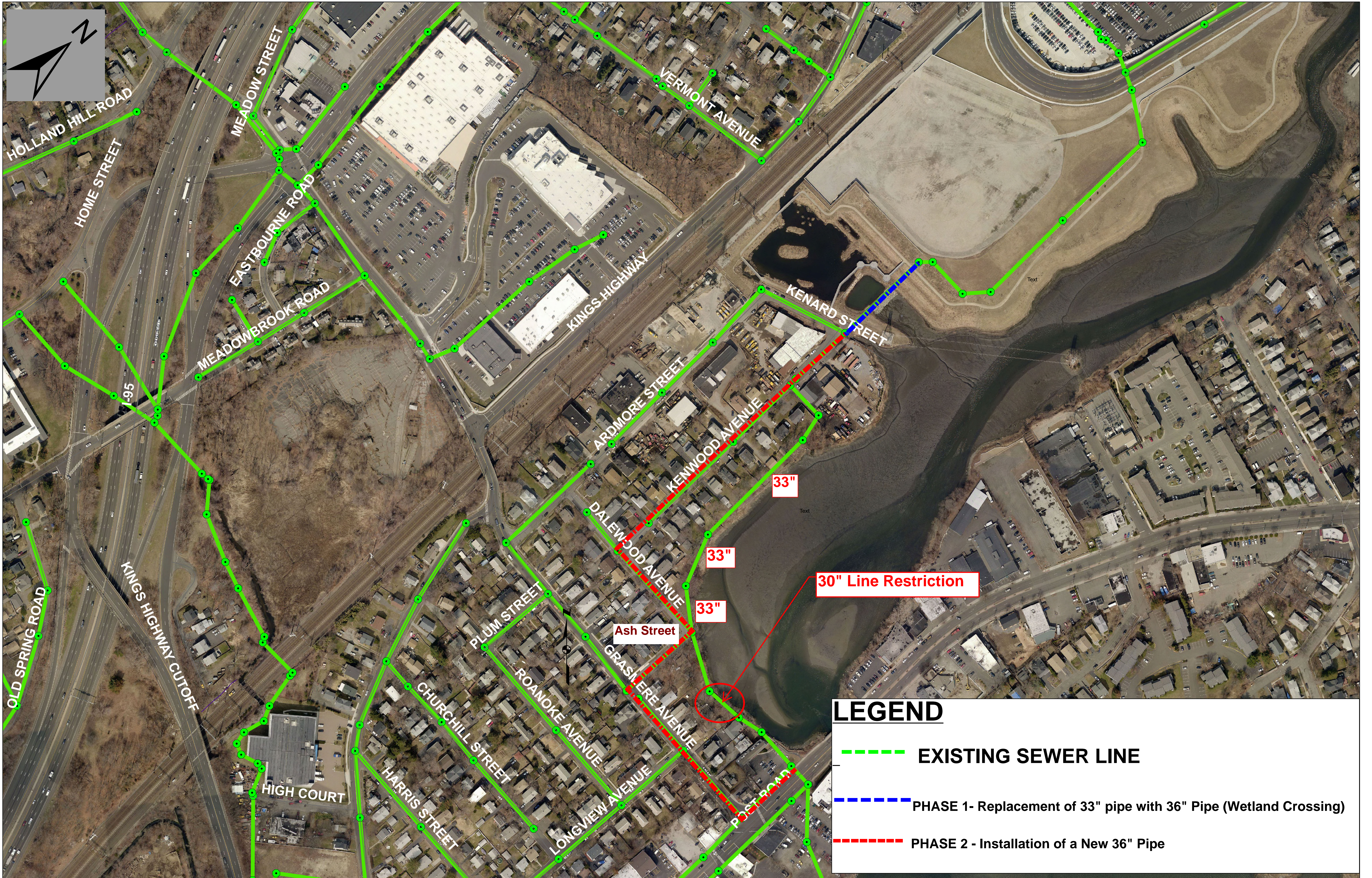
EAST TRUNK LINE INTERCEPTOR SEWER RELOCATION
