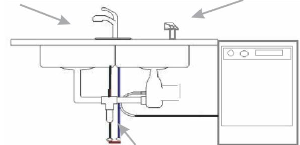
Hoses and water treatment devices may create a potential backflow hazard if not properly isolated with backflow prevention methods.
