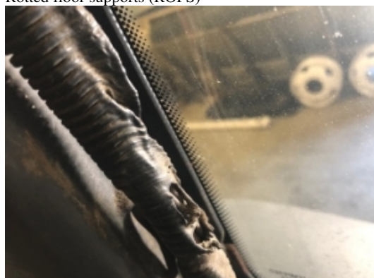
Melted wiring inside cab
