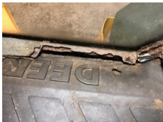
Rotted floor supports (ROPS)
