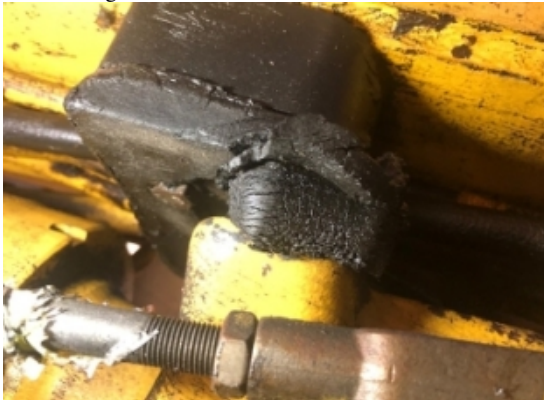
Isolator pad broken
