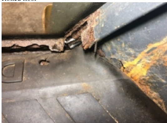
Rotted floor supports (ROPS)
