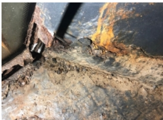
Rotted floor support (ROPS)
