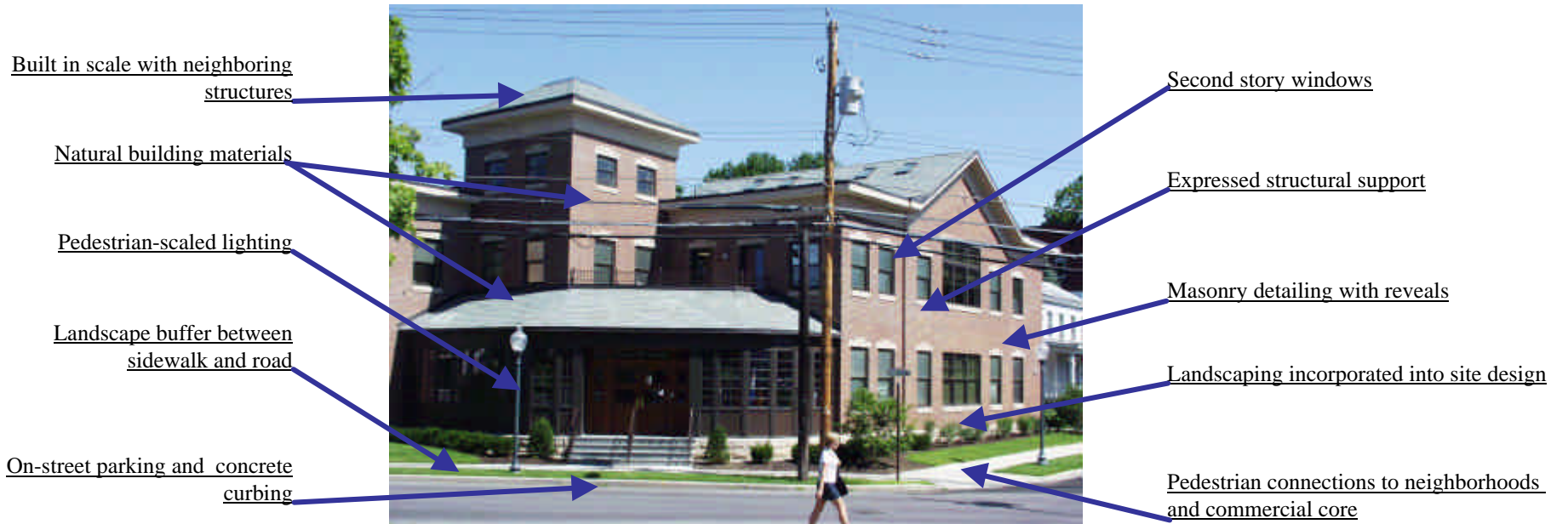
Example of a new light industrial building blending into small-scale urban environment
