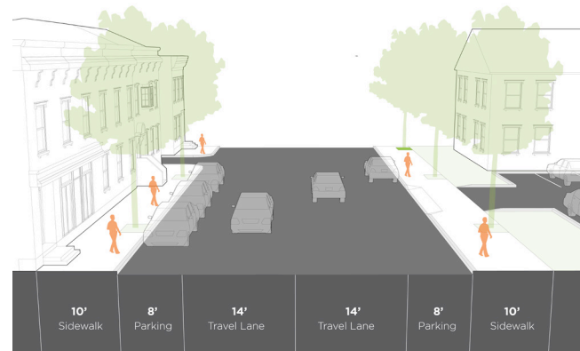
EXISTING SECTION LOOKING SOUTH ON FRONT ST.
