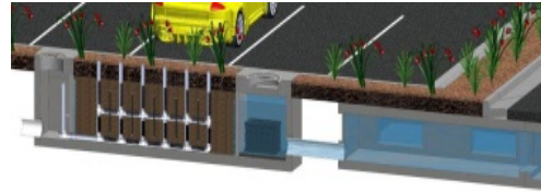
Horizontal Flow Biofiltration System
