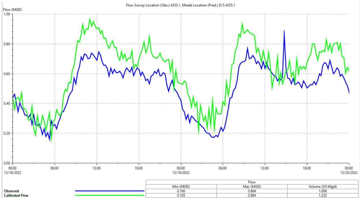
Figure 5.5 Example DWF Calibration Graph for Flow Meter 16
