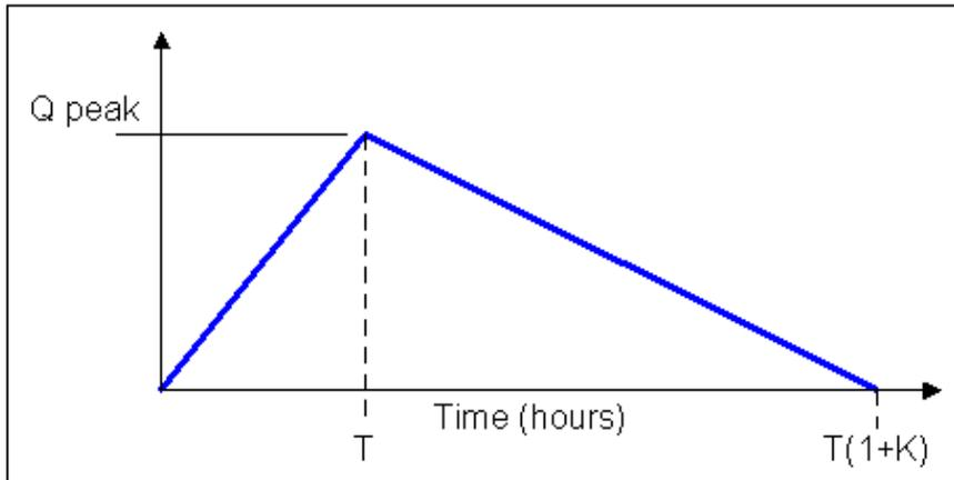
**Figure 5.3 Basic Parameters of the Triangular RTK Hydrograph<sup>2</sup>**
