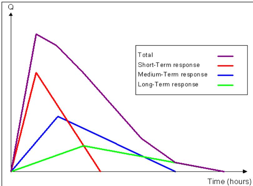
Figure 5.4 Fast, Medium, and Slow Components RTK Hydrograph<sup>2</sup>
