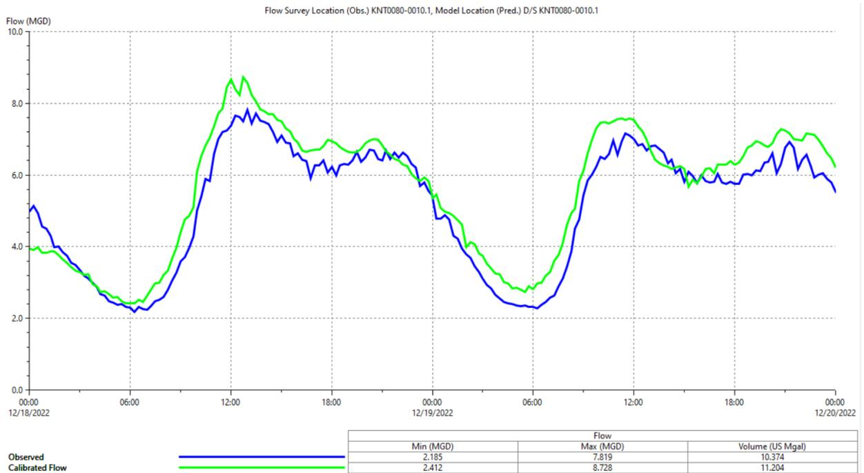
Figure 5.6 Example DWF Calibration Graph for Flow Meter 23
