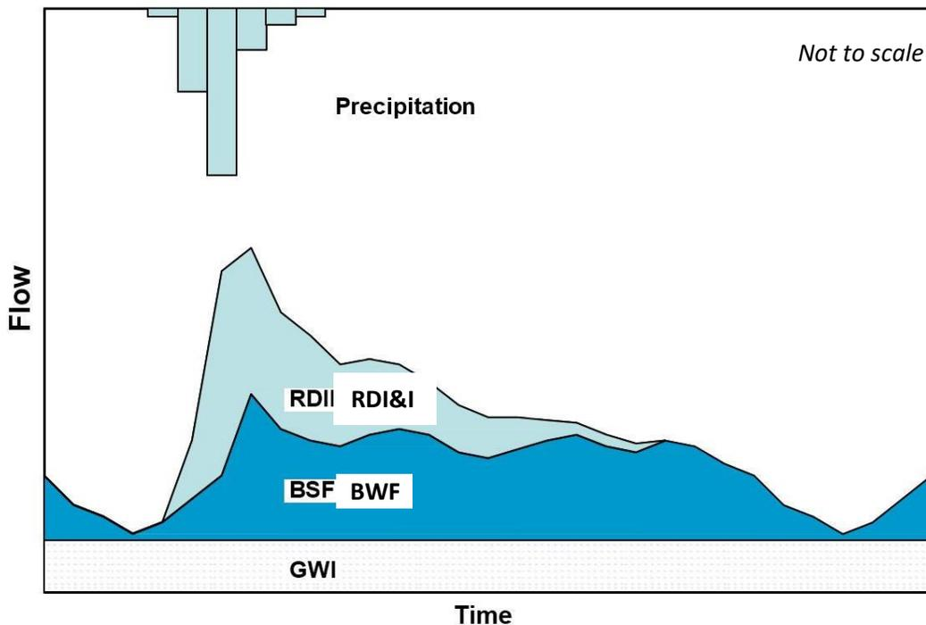
Figure 5.2 Components of Sanitary Sewer Flow<sup>1</sup>
