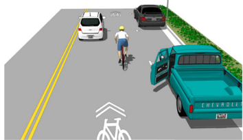
Wide Travel Lane - Shared with Cyclists Door Zone 7'-10' Parking Lane 11' minimum
