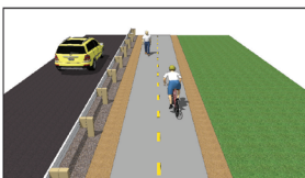
The edge of a bike path that is less than five feet from a road must have a physical barrier such as rails, dense shrubs or trees. (Caltrans Chapter 1000)
