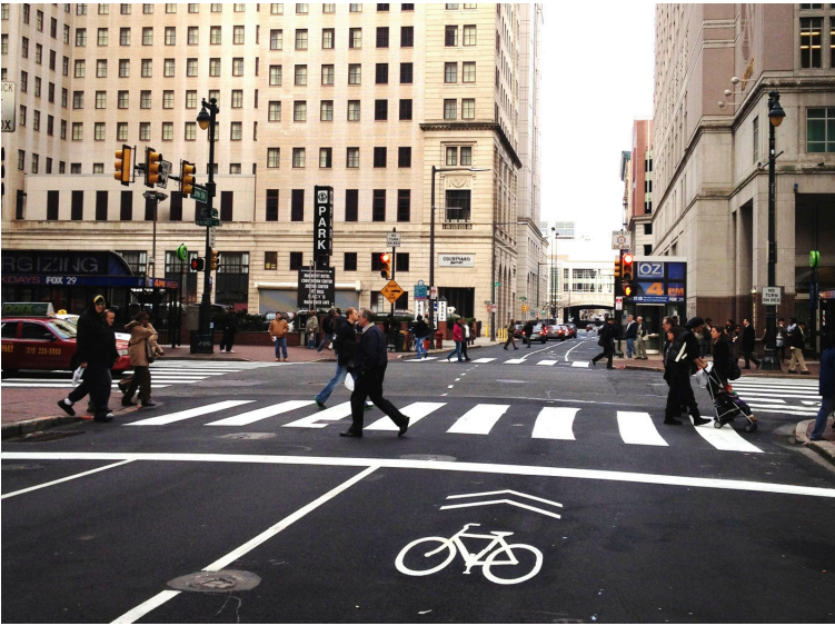
13B) Example of Shared Lane Marking directing cyclists through intersection - Philadelphia, PA (Photo credit: City of Philadelphia)
