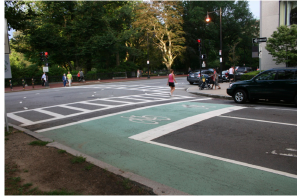
7B) A bike box creates an advanced stop bar for cyclists. This extra room provides an area for cyclists to cue up in front of vehicles waiting at red light. While this treatment is still considered experimental by the MUTCD, it is thought that it increases a cyclist's visibility, and therefore safety - Cambridge, MA
