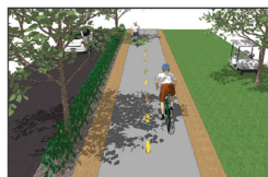
The edge of a bike path that is less than five feet from a road must have a physical barrier such as rails, dense shrubs or trees. (Caltrans Chapter 1000)
