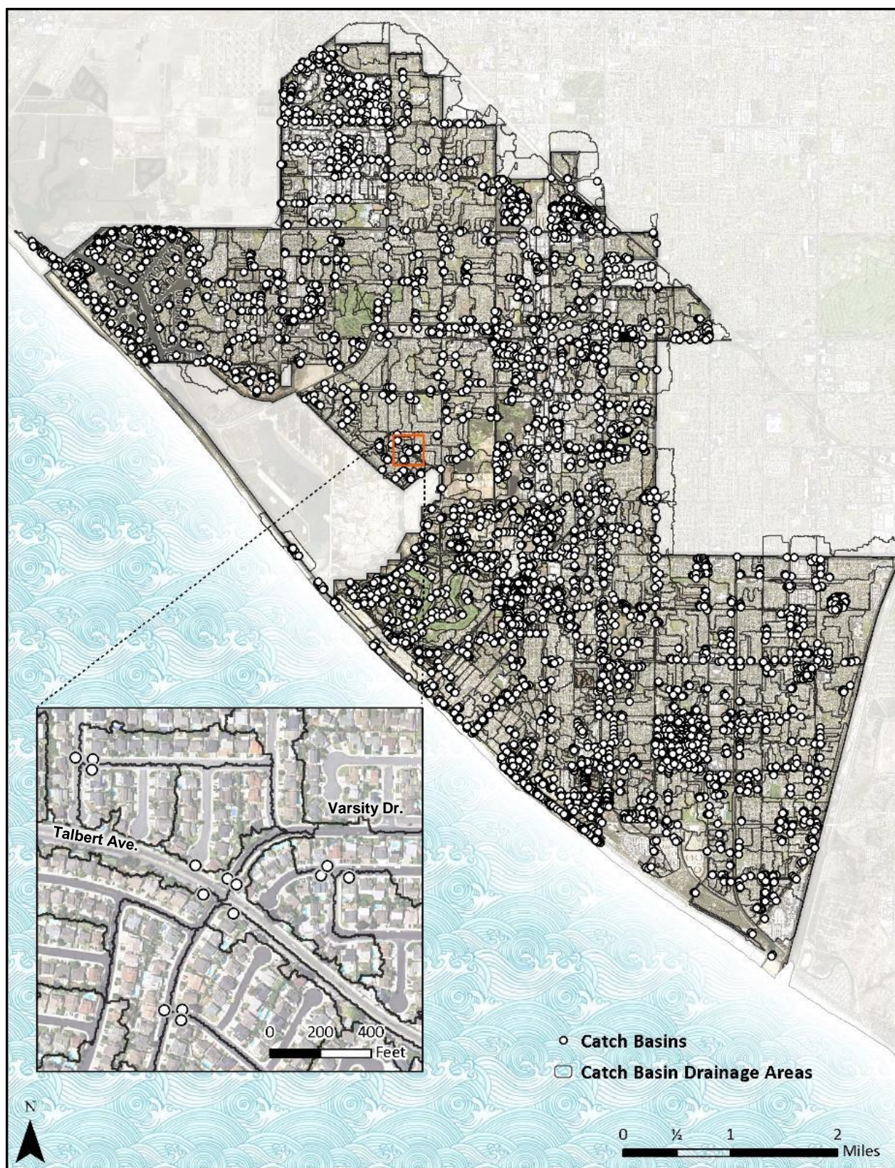
Figure 3-2. Location of all delineated drainage areas draining to their respective inlet node
