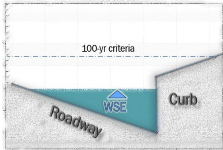
Figure 3-11. Conceptual cross-section of street flow conduit illustrating 100-yr, 24-hours storm criteria
