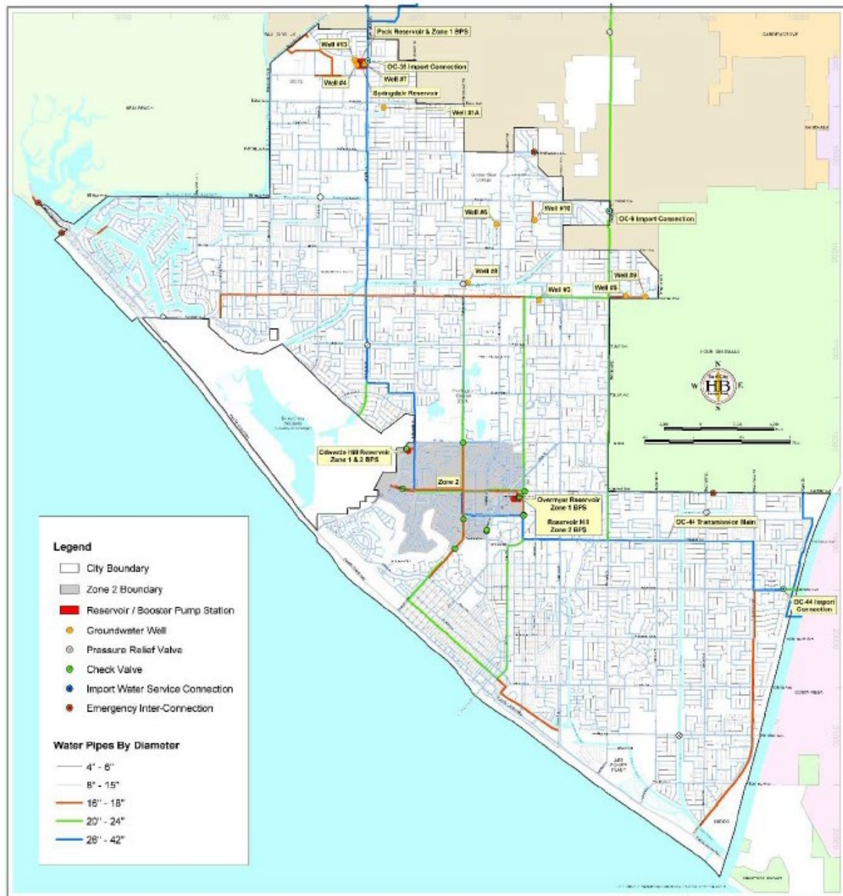
Figure 4-1 Existing Potable Water System Facilities
