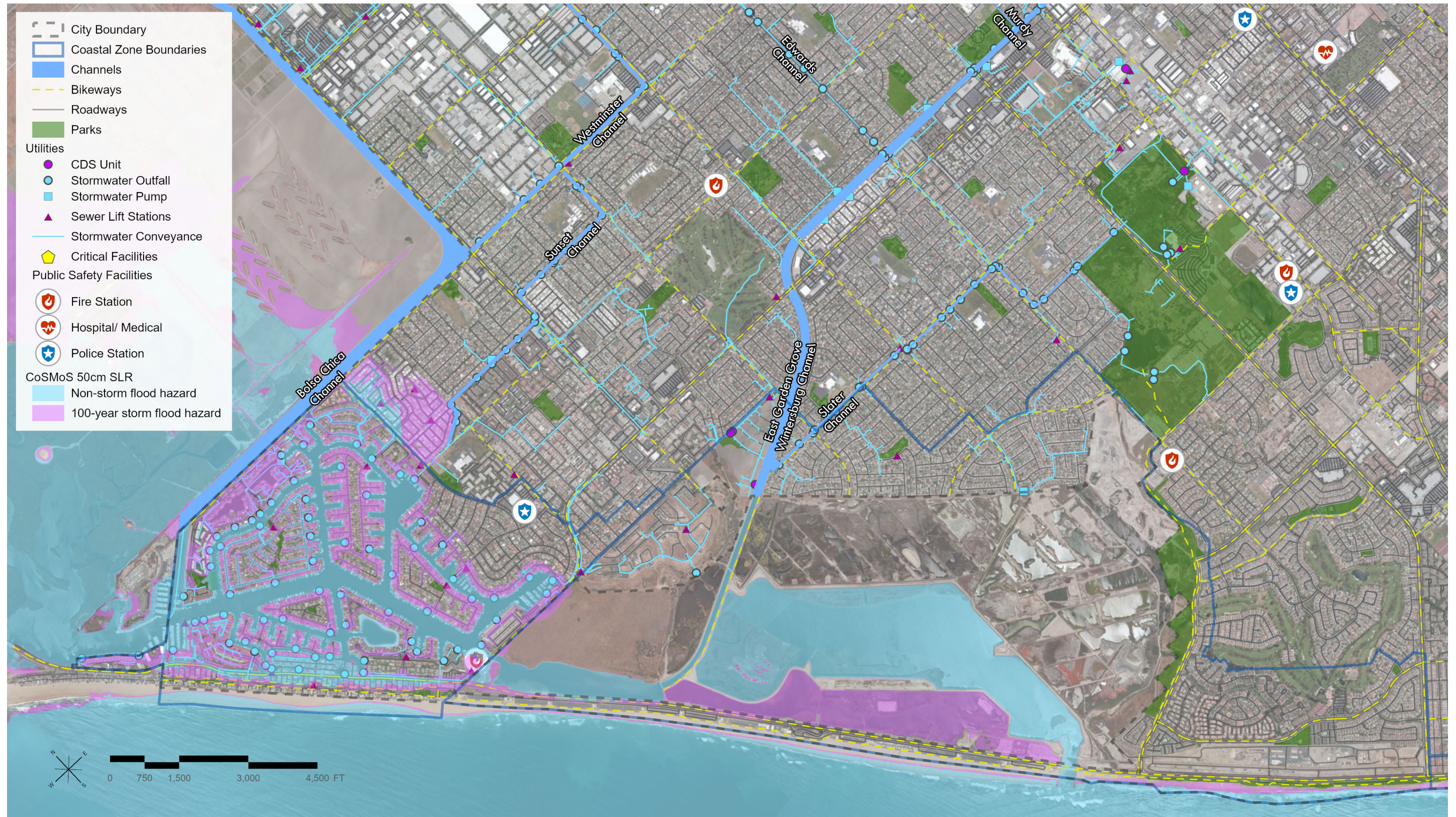
FIGURE 6-3: 1.6FT SLR HAZARDS, NORTHERN STUDY AREAS
