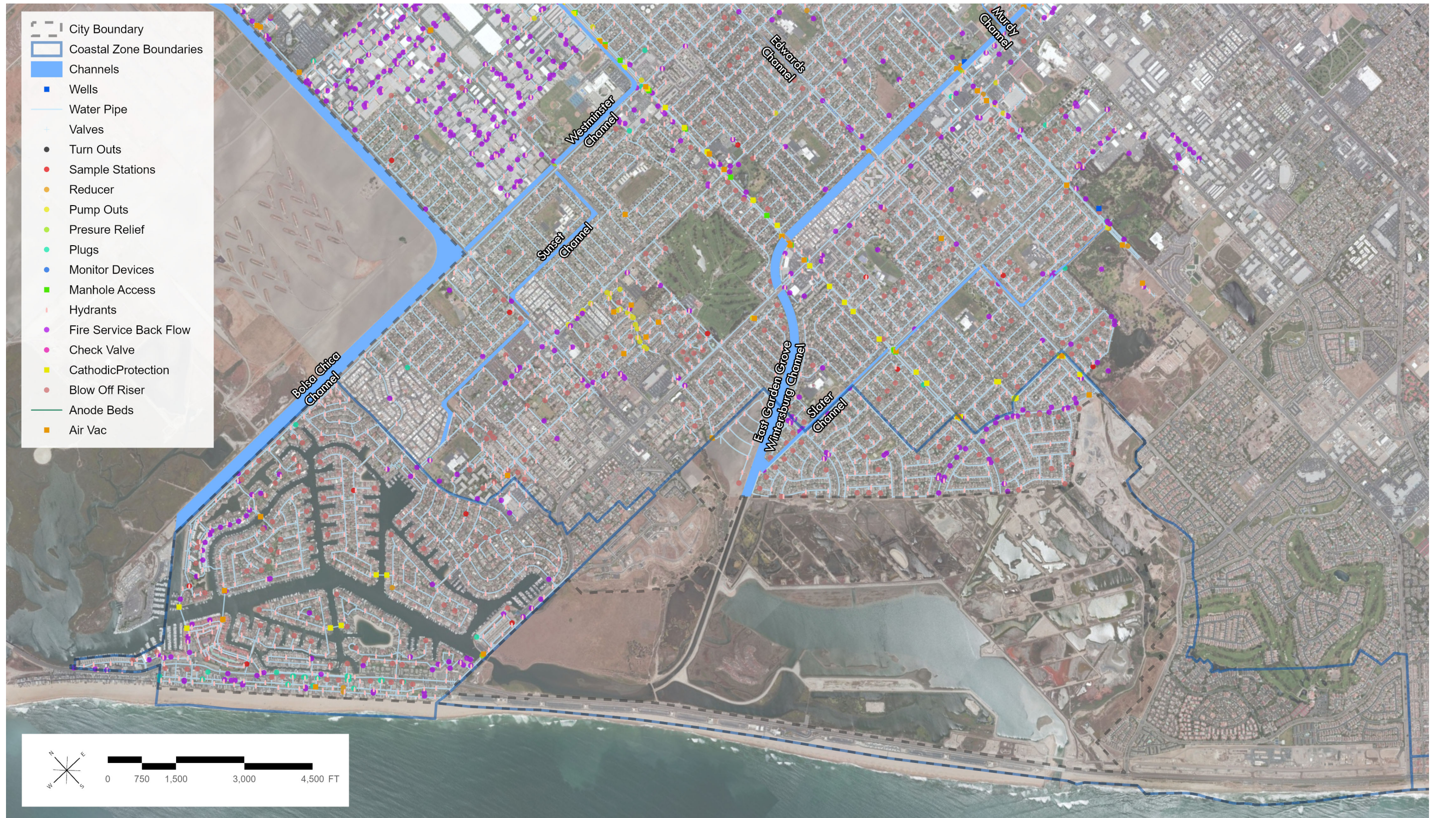
FIGURE A-1: POTABLE WATER INFRASTRUCTURE WITHIN POTENTIAL FLOOD HAZARD AREAS, NORTHERN STUDY AREAS.
