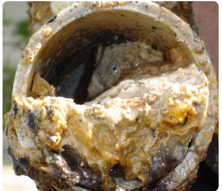
FOG Blockage in Sewer Pipe
