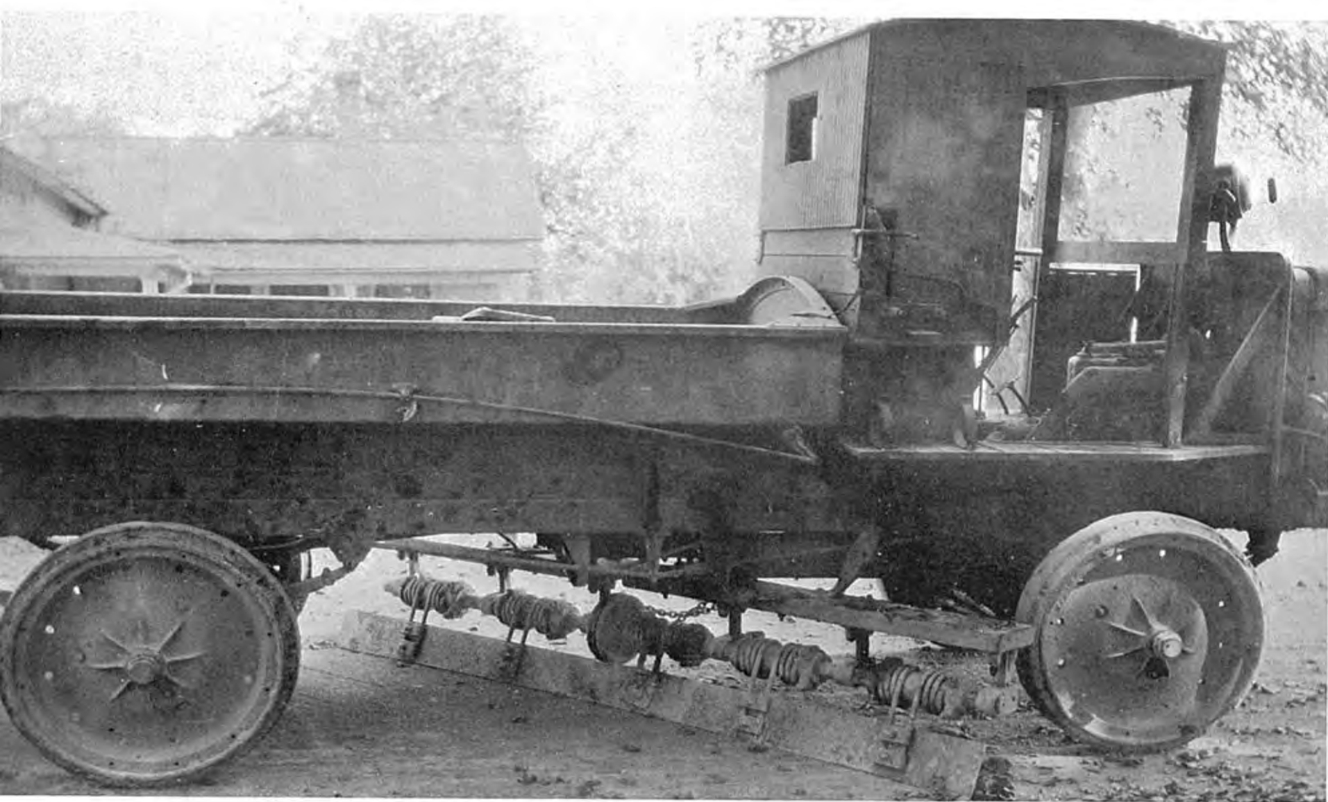
One of our truck-scraper outfits for maintaining gravel roads. This type of equipment saved us many thousands of dollars this season
