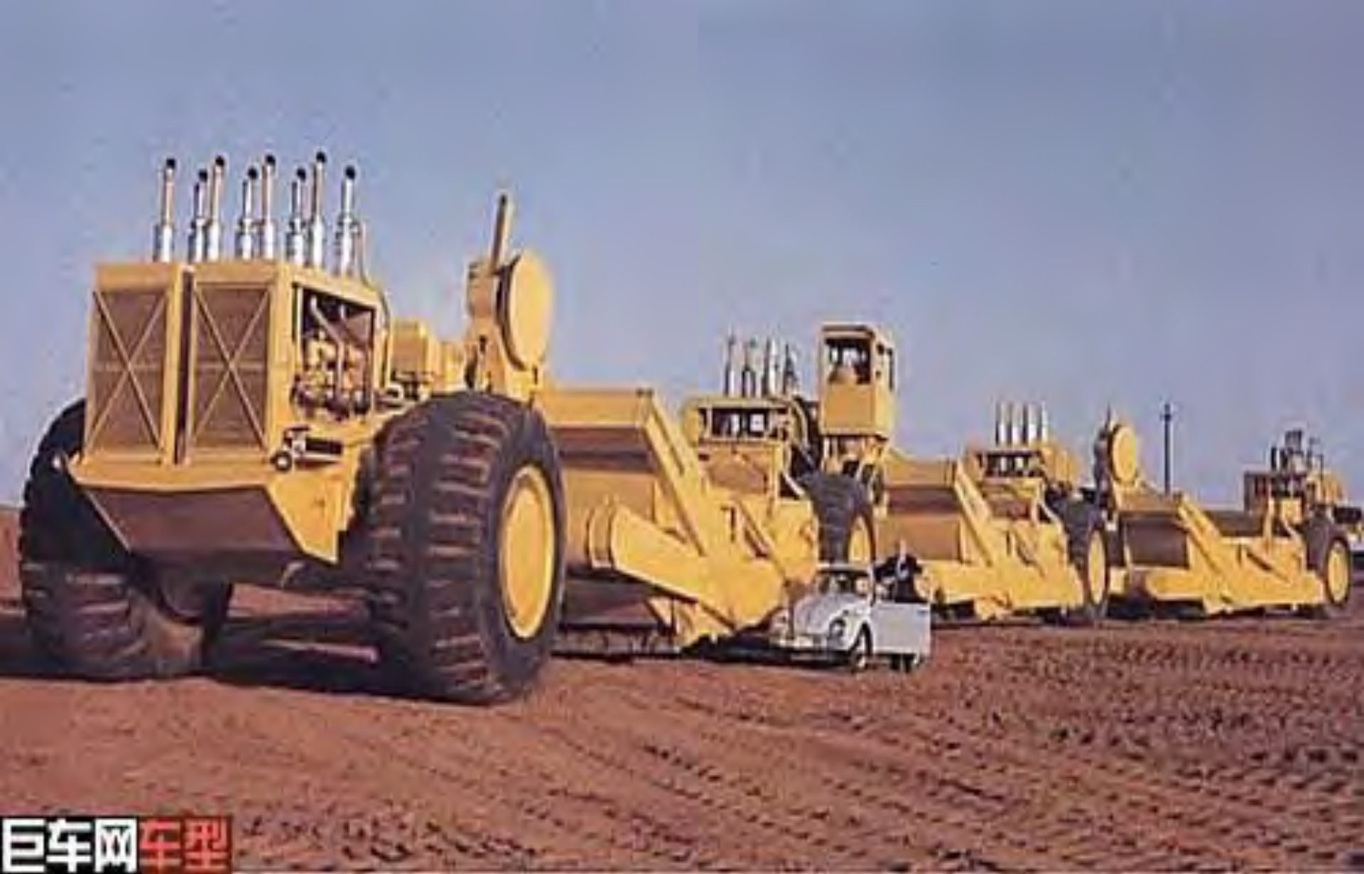
Close up of LeTourneau LT 360 8 Diesel 5080 Hsp 360 ton capacity
