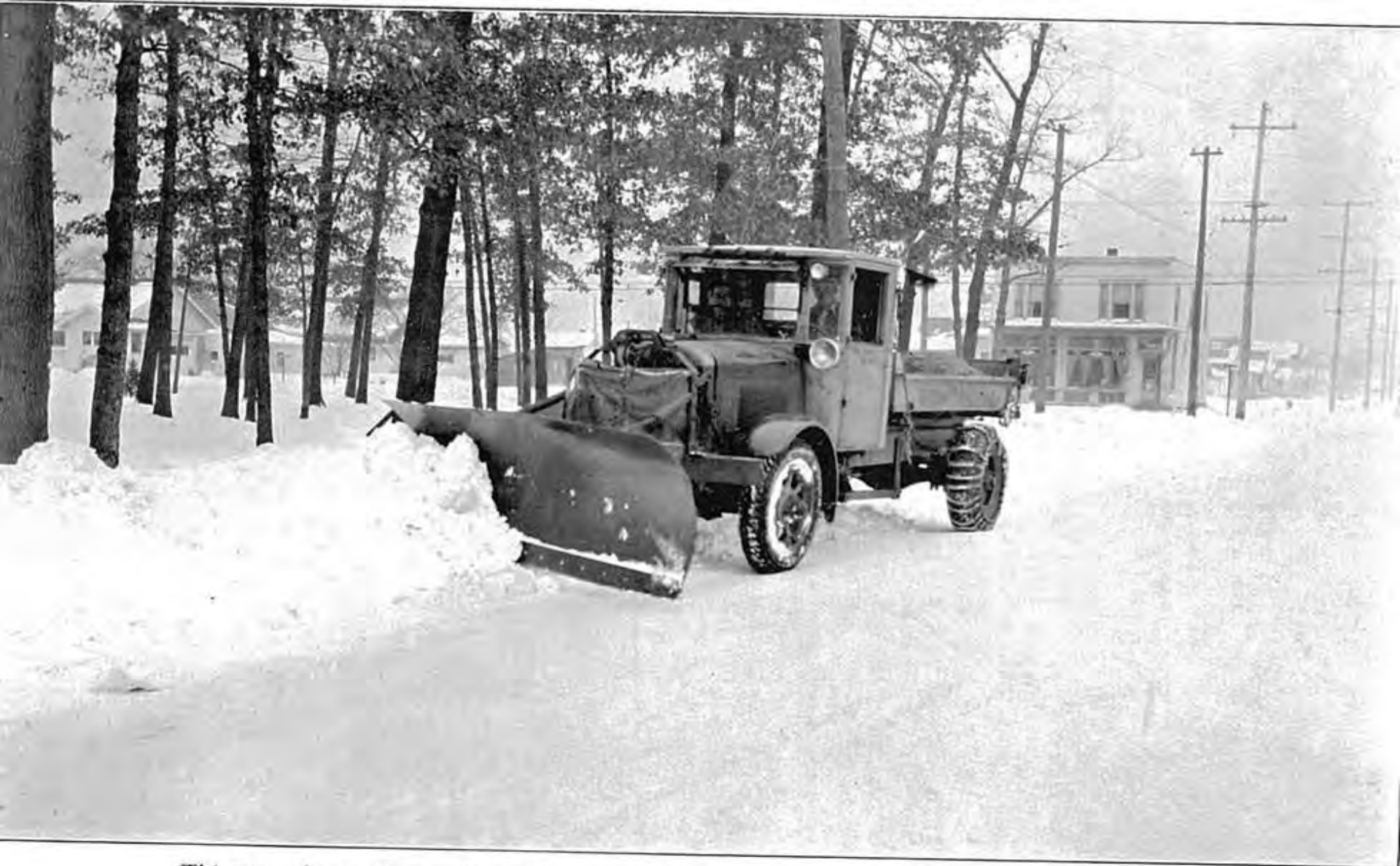
This type of snowplow equipment handles all of our snow removal work except very heavy drifts.
