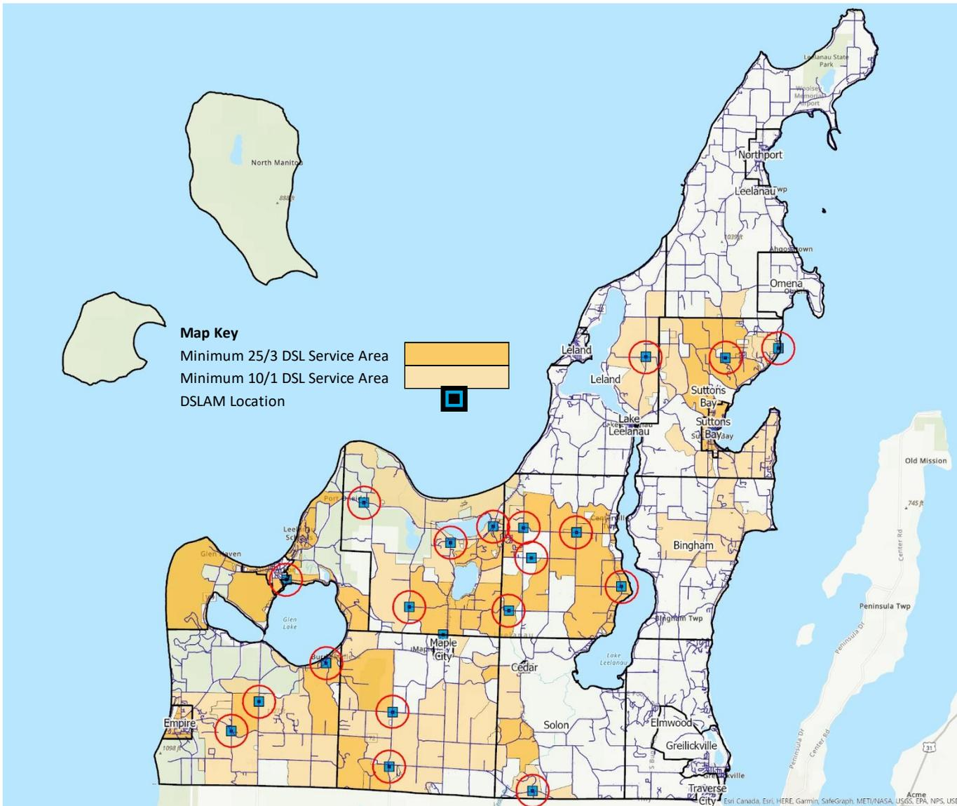
The DSL service areas are shown as reported by the two DSL carriers, and the DSLAM's were all located during the survey. The darker tan colored areas are the only areas expected to meet the FCC minimum of 25/3 based on reporting by the carriers.
