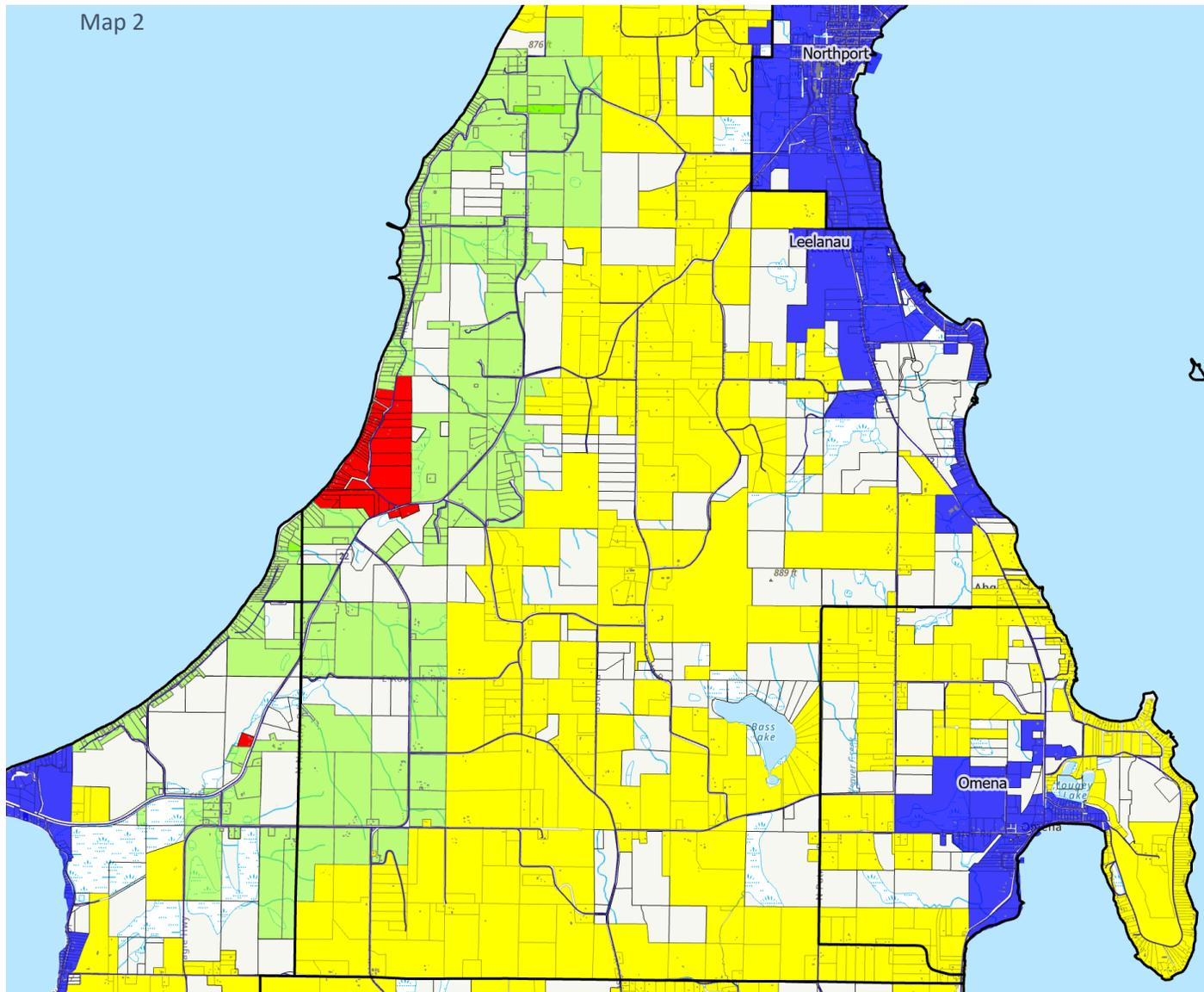
Cherry Capital Communications has also begun building fiber in their Gills Pier service zone. The red area is under construction, and the green area has been permitted for construction. It is assumed that the backhaul for this fiber area will be fiber since there are “Middle Mile” options near the main CCC node feeding this expansion. (Note, the data on this map was collected in June of 2021, so may be outdated. Look for updates on Cherry Capitals web site.)
