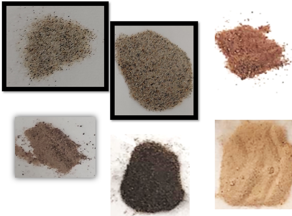
Figure 13. Photographs of ground samples. Clockwise from the top left, dune sand, beach sand, sand produced from ground red granite (albite), black sand produced from muscovite, white sand contained calcite, and other calcium-containing minerals.
