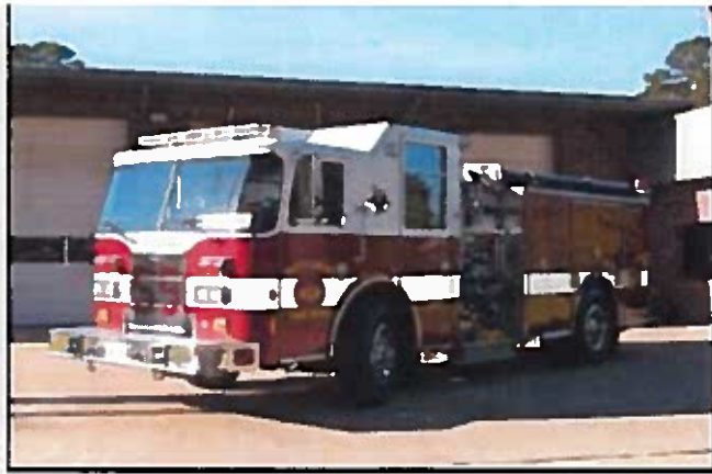
Engine 55 2007 Pierce Saber Pumper 1000 Gallon Tank 1250 GPM Pump
