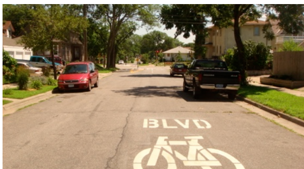
Pavement markings help communicate that bicycle riders will be also be using the street for their travel.
