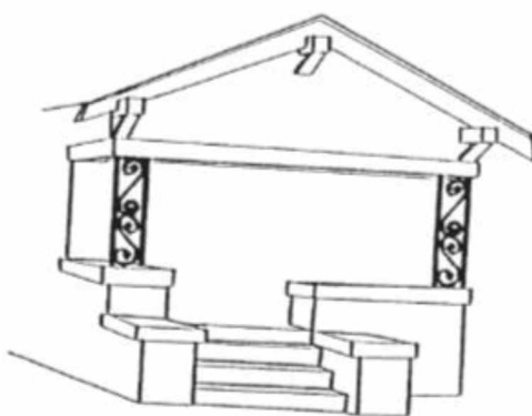
Inappropriate: wrought iron porch posts detract from the historic appearance of the porch
