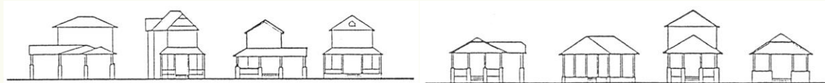
Appropriate: height and width consistent with neighboring houses. Porch and hipped roof break down height and mass of building.
