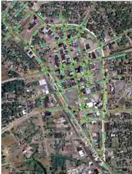
Traffic modeling software, including Synchro (shown above) and Vissim, was used to evaluate the existing traffic conditions as well as the traffic impacts of the various proposed alternatives.
