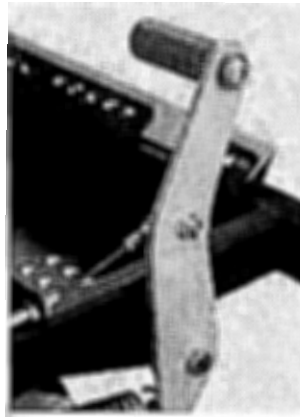
Cutter-deck-lift foot pedal is spring-assisted and makes raising the cutter deck smooth and easy.
