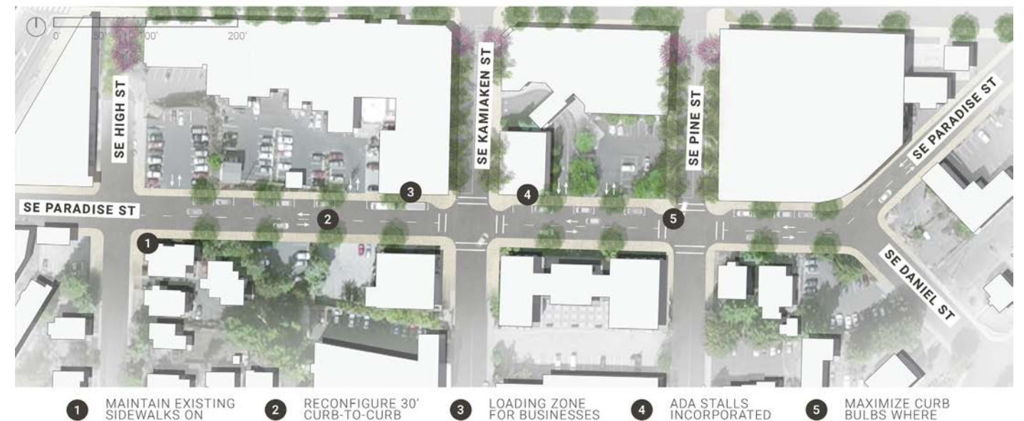
Figure 20. SE Paradise St after improvements, Framework, 2019
