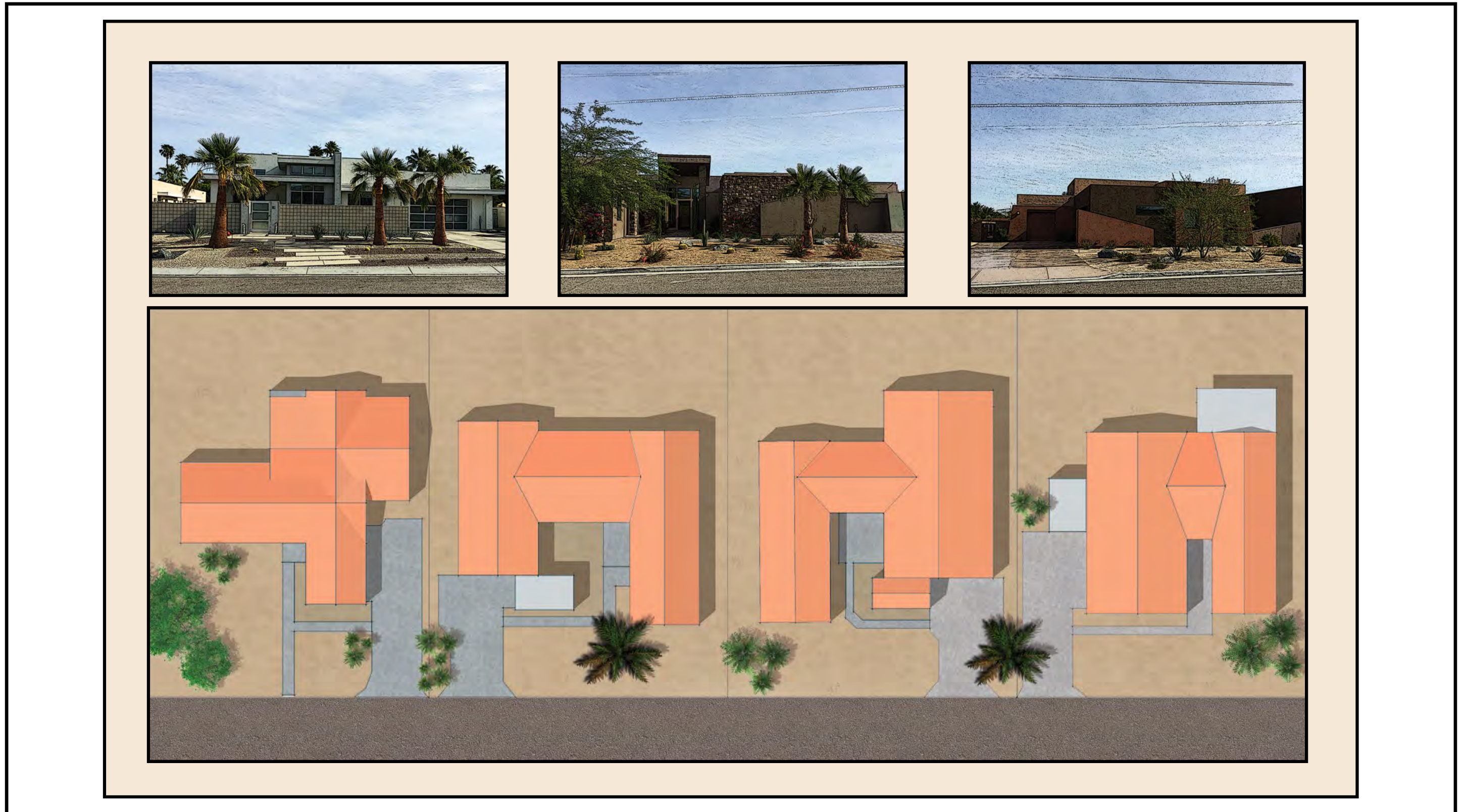
Exhibit 37 Example of Housing Development with Varying Setbacks, Garage Orientations, and Floor Plans.
