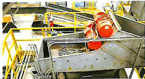
4: A series of screens are used to extract other contaminants.
