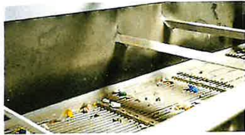
2: Quality Control: A vibrating finger-screen separates small pieces from large so contaminants can be easily removed by hand.
