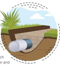
In cases of extreme rain events, French drains also have an outlet that drains out into a bubbler box, a device designed to hold excess rainwater that is unable to soak into the ground to be released through the surface. Many homes employ French drains to protect basements and levels of the house that are located below street level.
