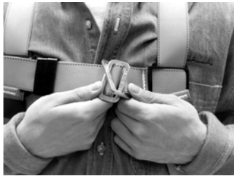
Figure 13A - Delta Vest™ Harness Buckle Connections
