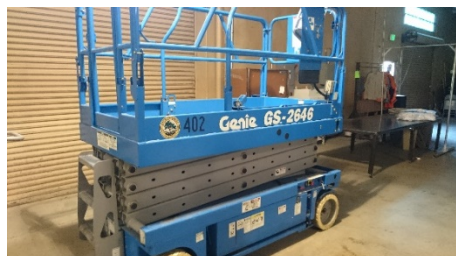
Figure 1. Elevating work platform (scissor lift) Genie GS-2646, 26' max.
