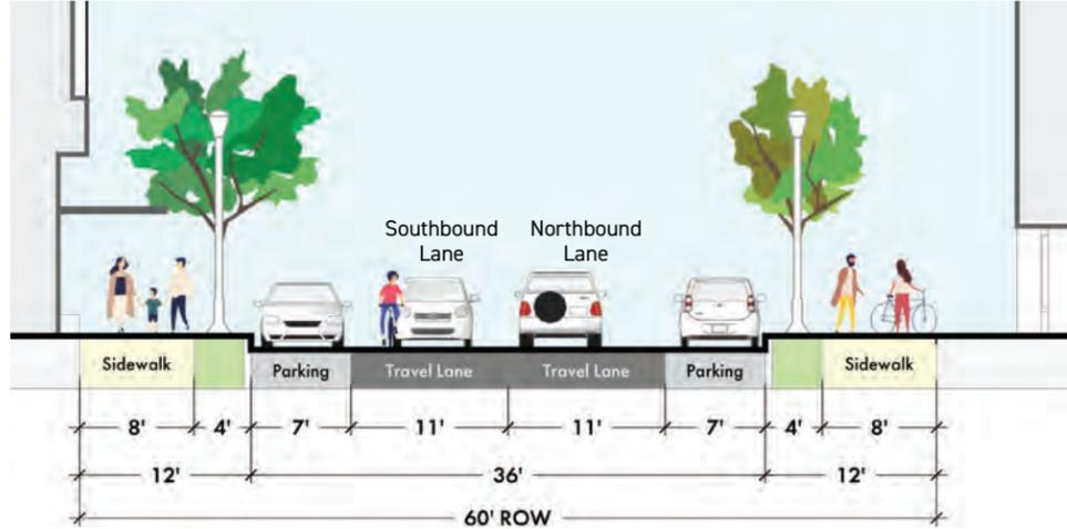
Fig. 79: Proposed Typical Street Section
