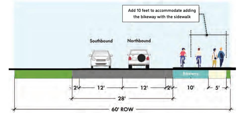
Fig. 95: Proposed Section: Riverside Drive Multi-use Trail
