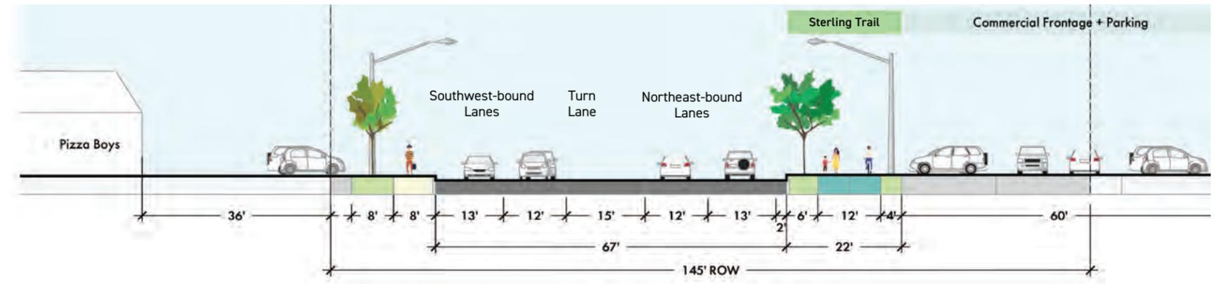
Fig. 99: Proposed Section AA: Sterling Highway Multi-Use Trail
