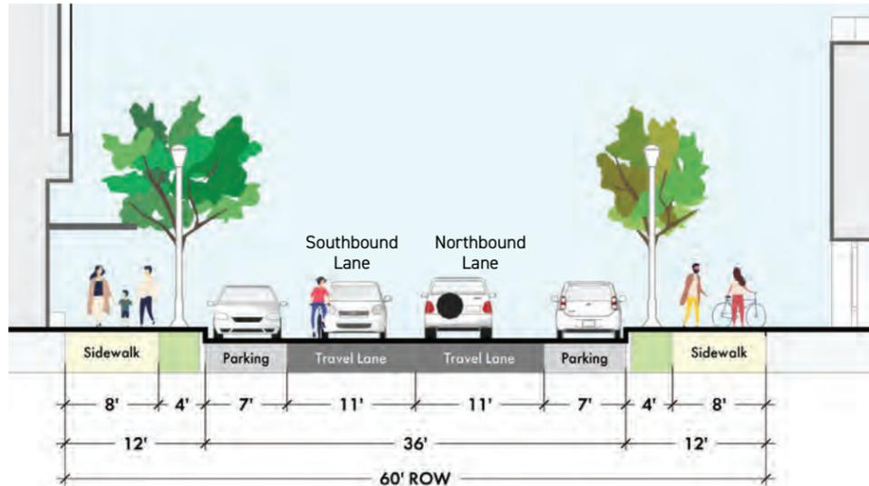
Fig. 76: Proposed Typical Enhanced Street Section
