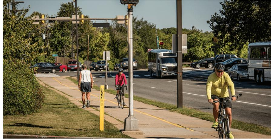
Fig. 96: Multi-use Trail with Buffer on Multi-lane Arterial Roadway
