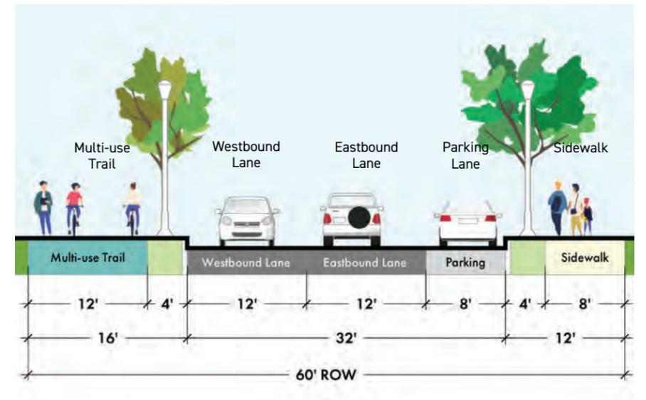
Fig. 74: Proposed Typical Enhanced States Avenue Section
