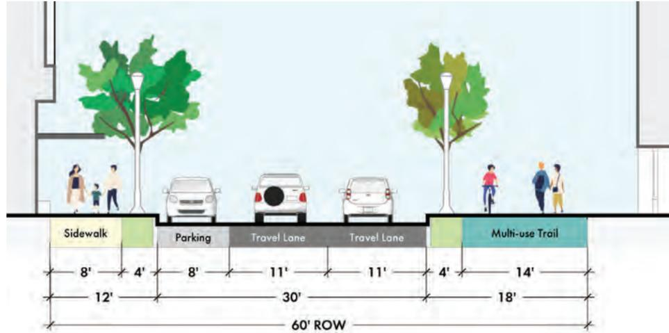
Fig. 80: Proposed Typical Street Section w/ Multi-Use Trail
