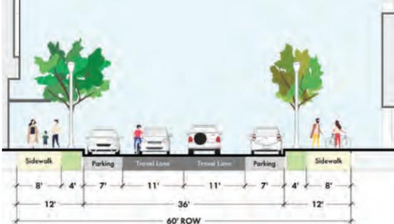
Fig. 26: Street Grid- 60-foot Wide Right-of-way
