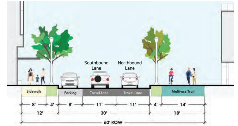
Fig. 78: Proposed Typical Enhanced Street Section w/ Multi-Use Trail
