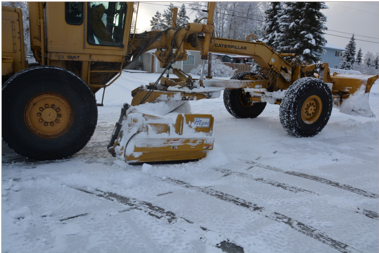
Figure 8 – City Grader with Driveway Gate in Action
