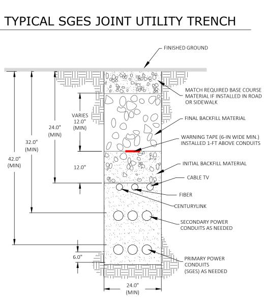
NOTE SHOWN BURY DEPTHS ARE TYPICAL; EXISTING BURY DEPTH MAY VARY FROM WHAT IS SHOWN. WHERE WALL CONSTRUCTION OR GRADING ADJACENT TO THE EXISTING JOINT UTILITY TRENCH OCCURS, CONTRACTOR SHALL FIELD VERFIY BURY DEPTH WHILE SGES INSPECTOR IS PRESENT AND COORDINATE CONSTRUCTION METHODS AND TIMELINE WITH SGES WHILE WORKING IN THESE AREAS.
