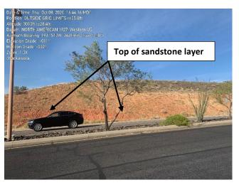
The lower portion of the slope is sand and sandstone bedrock (eastern portion) while the top of the slope is capped with basalt cap rock. The basalt is moderately fractured and granular. The sand is medium dense and slightly cemented. The sandstone bedrock is mostly on the eastern portion of the exposed slope as shown in the photos above.
