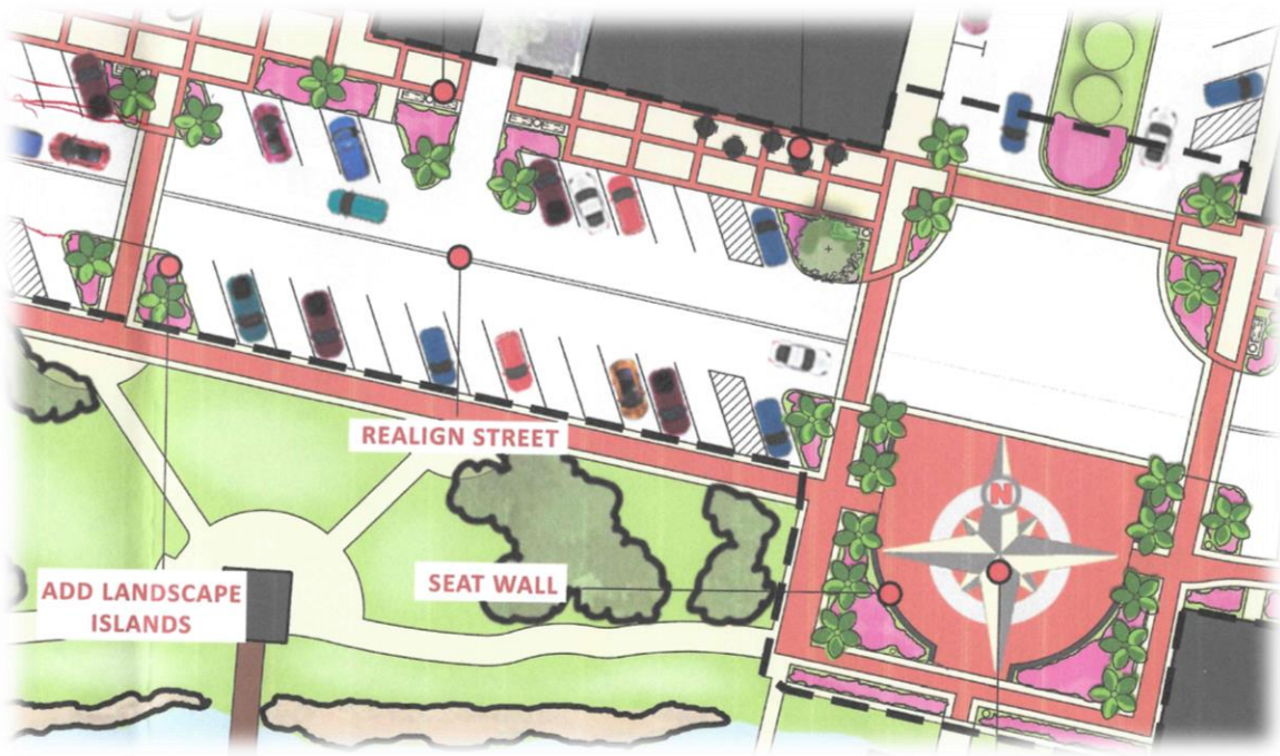
Concept Drawing of Sidewalk Hydrologic Redevelopment and Improvement Project (SHRIMP) with Bio-Retention Landscaped Islands, courtesy of Goodwin, Mills, and Cawood, Inc.
