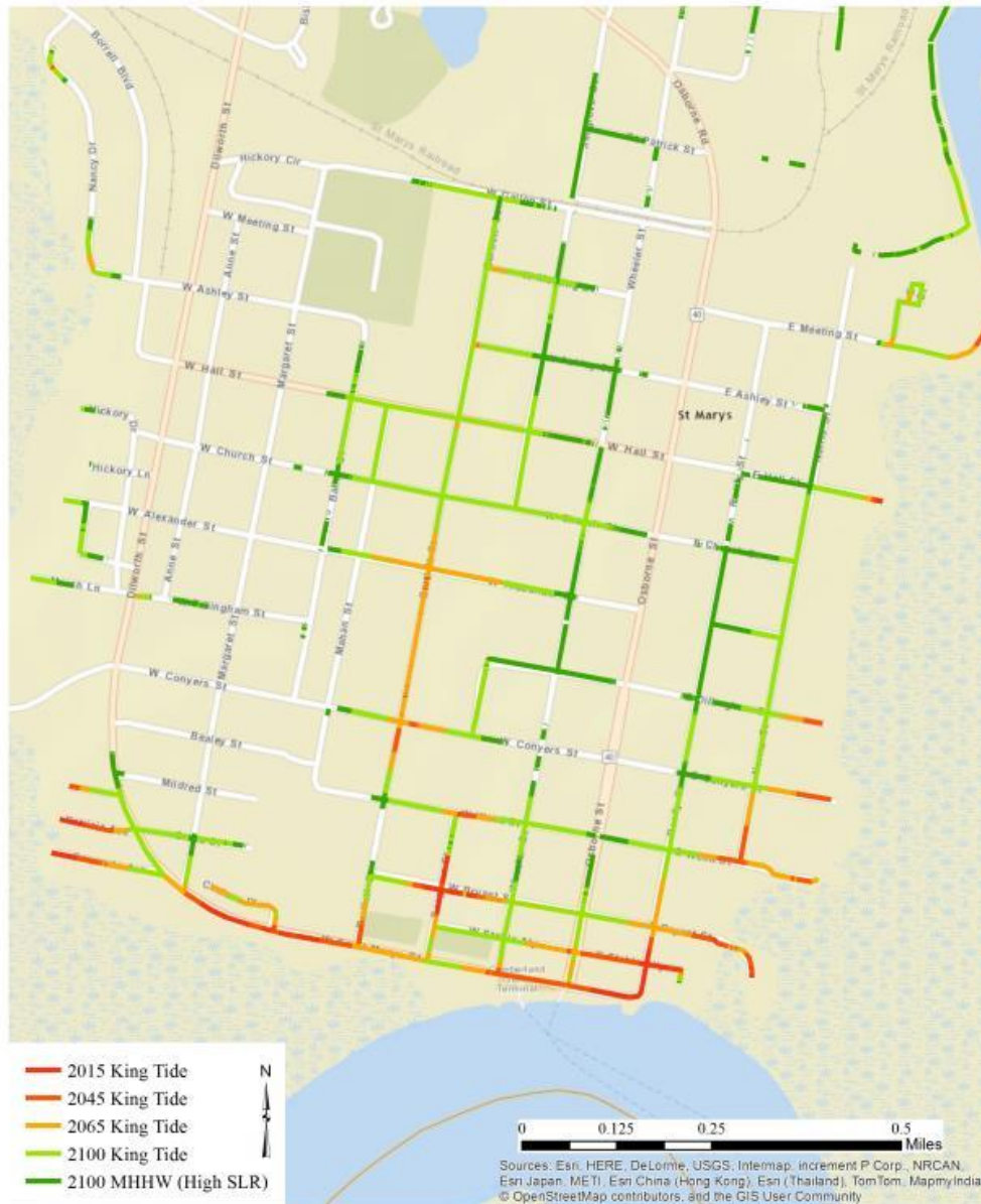
Figure 4.5: Close up of road segment vulnerability in downtown St. Marys, GA, to current and future king tides with Intermediate High sea-level rise
