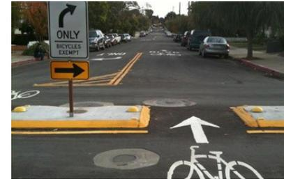
Enhanced crossing of arterial via median refuge traffic diverter
